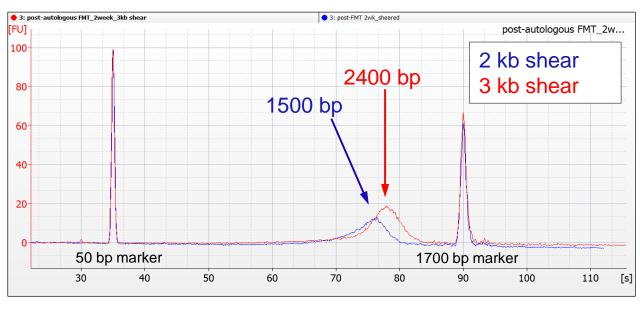
Figure 3. Bioanalyzer<sup>®</sup> traces of 2 kb and 3 kb shears, sample 3. Both shears were combined in the library for sequencing.
