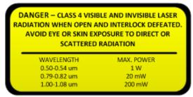
Do not operate the instrument with any of the panels removed. When the front door of the instrument is open, the laser beam is blocked via safety interlock switches. If you operate the instrument with any of the panels removed, you risk exposure to direct or reflected laser light.
