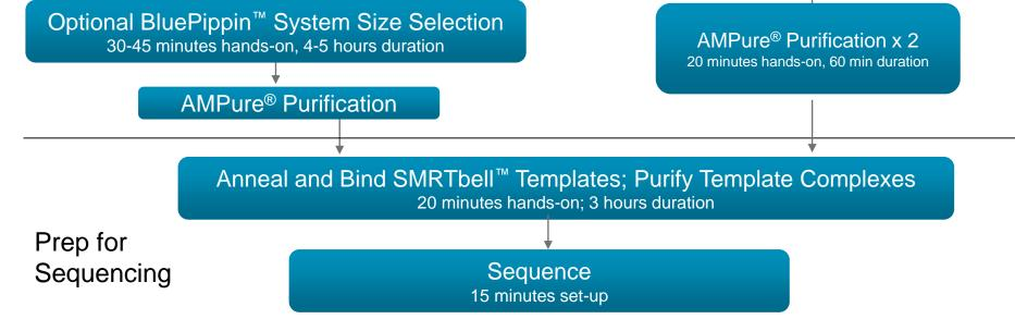
Steps in microbial multiplex barcoded library prep from input QC through sequencing set-up, including approximate hands-on and duration times. The entire process can be done in < 2 days, excluding size selection.
