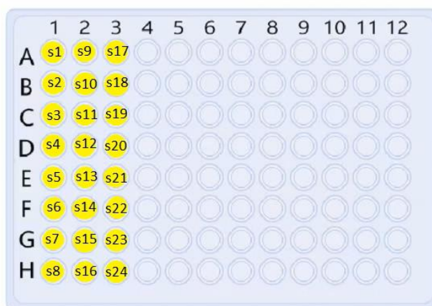
Figure 1. Sample input plate example for SRE for 24 samples (s1–s24). Prepare in a 96-well PCR 200 \mu L plate (PN: HSP9601).
