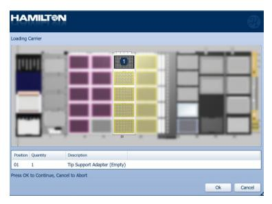
**13. Tip Deck Layout.** A prompt displaying the tip positions will appear, including the tip adapter position. There are 4 tip carriers. Refill the tips on deck in the positions for each tip size: 50µL filtered conductive tips, 300µL filtered conductive tips.
