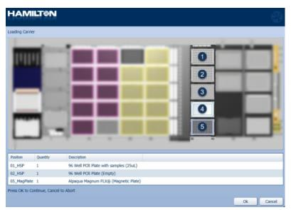
13. Load the Master Mix tubes on cold block. into the designated positions on the 4°C cold block adapter. The prompt is set for 96 samples. Click "OK" to continue.
