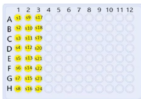
Figure 1: 24 sample input plate example (s1 – s24). Prepare in the 96-well PCR 200µL plate (Bio-rad, HSP9601).
