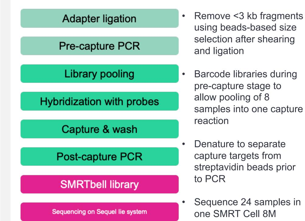
**Figure 2**. Workflow for sample preparation. Protocol and reagents from PacBio<sup>2</sup> used for steps in pink, Twist in green, and third party in grey.
